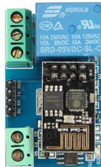
Figure 2. ESP 8266 chip with relay
